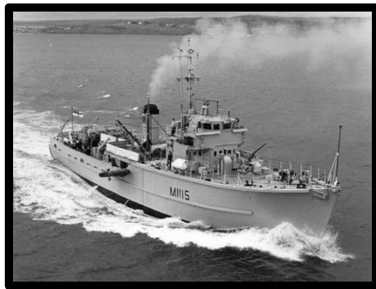
HMS BRONINGTON is one of around 120 Ton-class minesweepers built in the 1950s. With hulls of mahogany, the TONS were the last wooden warships built for the Royal Navy before it switched to today's plastic-hulled Mine Hunters (HUNTS and SANDOWNs) in the 1970s. (More ship details, [here](#)).
